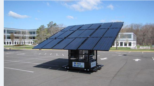
Figure 1. Solar-powered Water Purifying Pump
